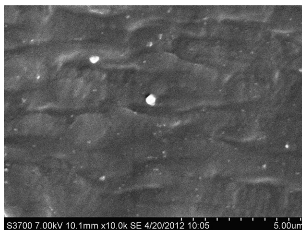
Figure 9. SEM photograph of the fracture surface of the PCL/nano- \text{CaCO}_3 composite ( \phi_f = 3\% ).
